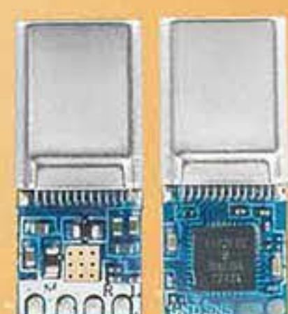
KT02F20/KT02H20 采样率: 96KHZ/384KHZ
